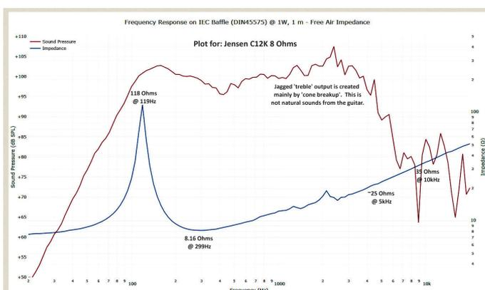
You can also see a huge spike at 119Hz where the speaker's impedance rises to 118 Ohms. At this point, the speaker's cone is at resonance. This resonance produces huge output for a relatively small amount of input power to the speaker... and this is where a tube amplifier's 'warmth' comes from. Actually, nothing to do with the properties of valves as claimed.
