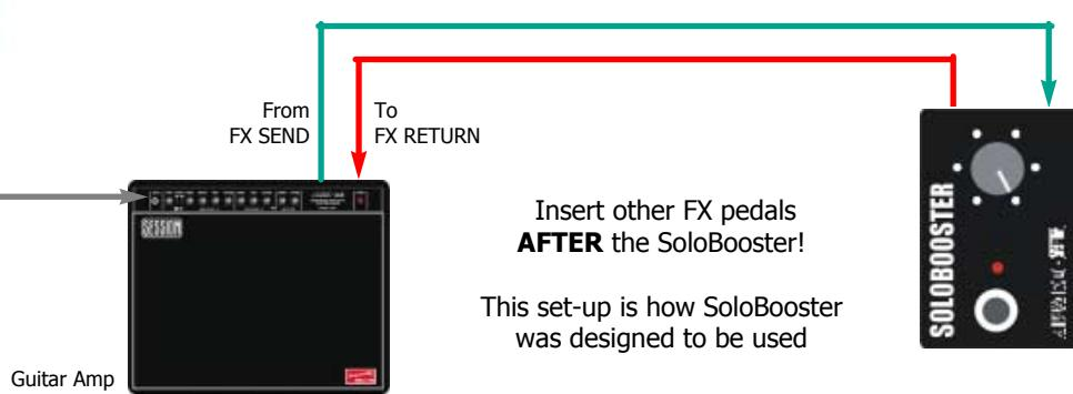
**SoloBooster™** is a handy footswitchable MASTER VOLUME control that can be used to lower the volume of your soloing sound for use behind a vocal. This 'background' volume can be set with the LEVEL control. Then, when it's time for your solo, you just step on the footswitch for full-on solo volume - easy!
