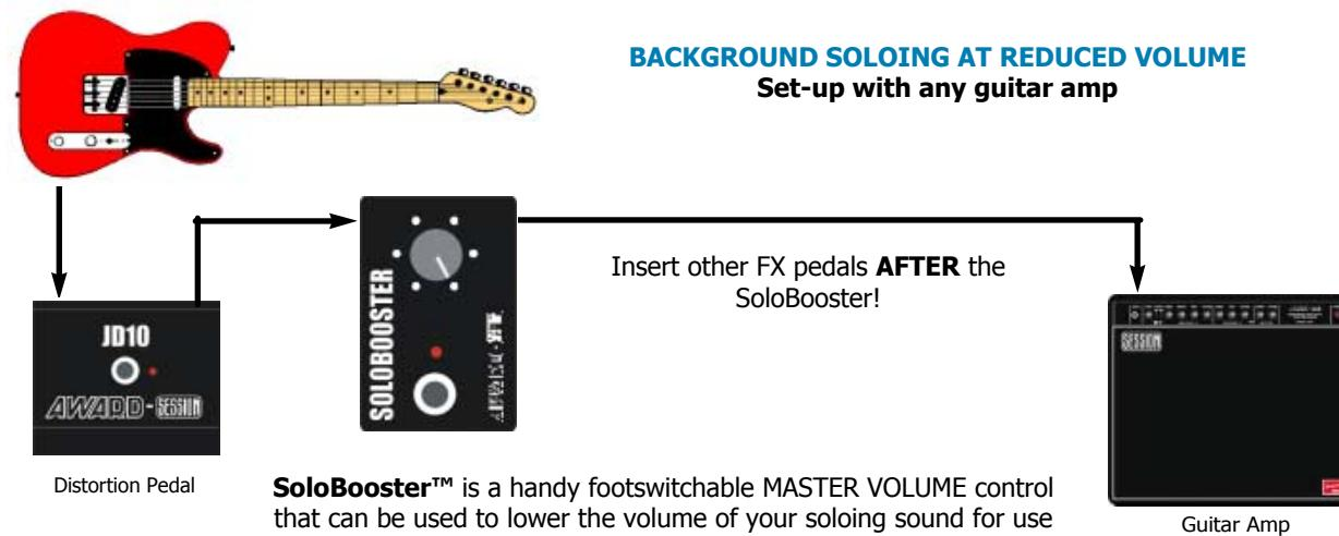
**SoloBooster™** is a handy footswitchable MASTER VOLUME control that can be used to lower the volume of your soloing sound for use behind a vocal. Then when it's time for your solo you just step on the footswitch for full-on solo volume - easy
