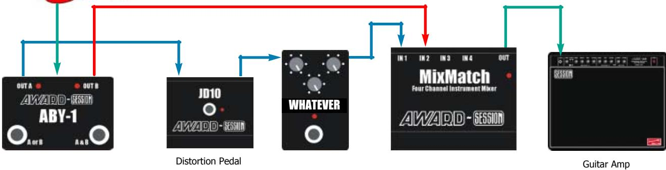
**ABY-1** is a high quality signal switcher using robust latching footswitches. Use it to switch your guitar between two signal paths - effectively creating two EFFECTS LOOPS. Why not insert a chorus or flanger into the RHYTHM line? The A&B switch allows both channels to operate simultaneously
