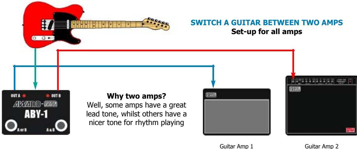
**ABY-1** is a high quality signal switcher using robust latching footswitches. Use it to switch your guitar between two amps. You can insert different effects pedals into each of the two signal paths too!
