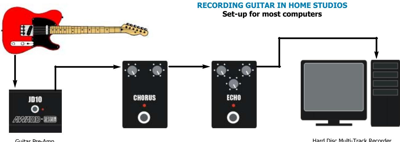
JD10's selectable **G12T Speaker Simulation** means it can be used as a pre-amp for recording **direct to hard disc** or tape. Plug into the computer's LINE IN socket.
